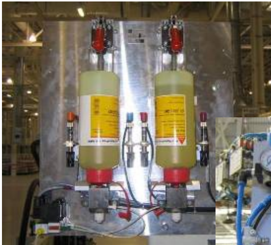
EcoGun Gluing S Process head for spray application
