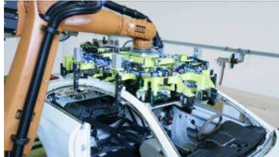
Roof module insertion
