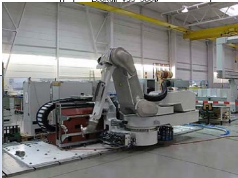
EcoRP L153, flexible 9-axis van painter
