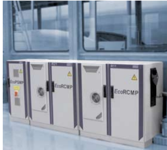
EcoRCMP and EcoPSMP for painting system with 2 robots (low version)
