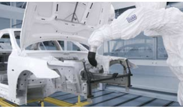
Interior painting station - hoods
