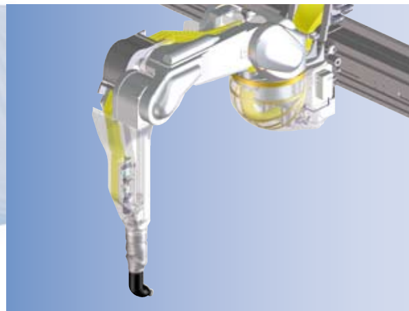
Hose guide through central seam of robot axis
