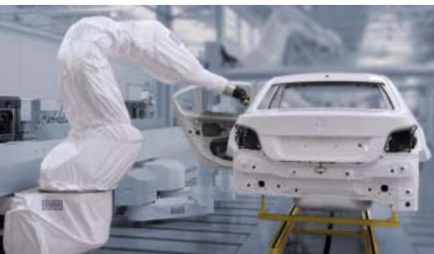
Interior painting station - doors
