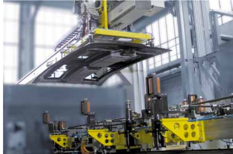
Gluing of roof module
