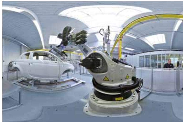
Gluing cell in the Ecopaint Testcenter Gluing
