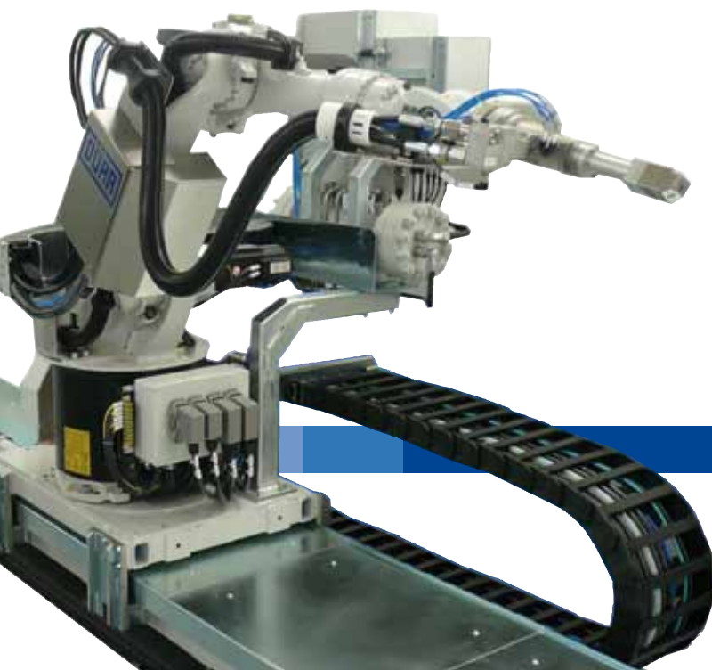
EcoRS robot with application equipment on EcoRail travelling axis
