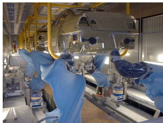
EcoRail HL with robots for seam sealing
