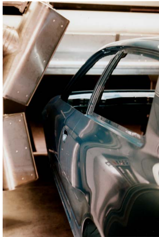
Nozzles at the side station
